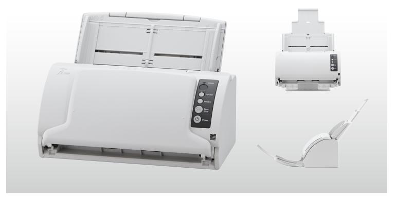
The fi-7030 scans A4 portraits at 27 ppm/54 ipm (200/300 dpi), loads up to 50 sheets at a time, and ensures efficiency with quick startup times and a small footprint.
